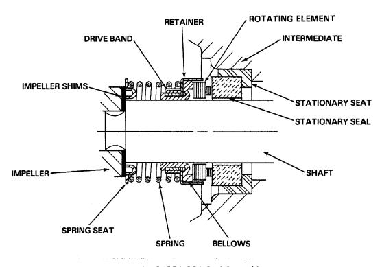
Figure 2. 25271-821 Seal Assembly
