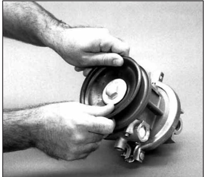
Step 10: Using an adjustable wrench, or by rotating the diaphragm by hand, remove the diaphragm assembly from the center section.
