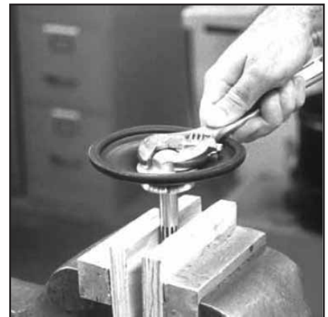
Step 12: To remove the diaphragm assembly from the shaft, secure shaft with soft jaws (a vise fitted with plywood or other suitable material) to ensure shaft is not nicked, scratched, or gouged. Using an adjustable wrench, remove diaphragm assembly from shaft. Inspect all parts for wear and replace if necessary.
