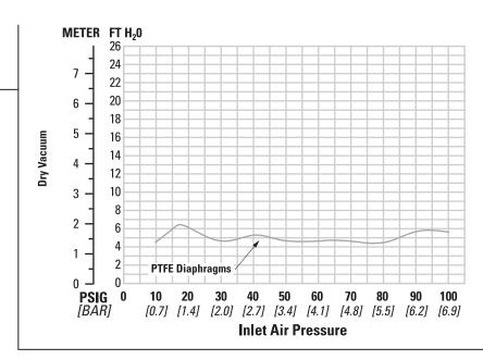
Suction lift curves are calibrated for pumps operating at 305 m (1000') above sea level. This chart is meant to be a guide only. There are many variables which can affect your pump's operating characteristics. The number of intake and discharge elbows,
