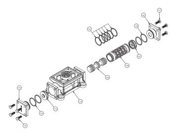
Valve Assembly for Aluminum Mid Sections
