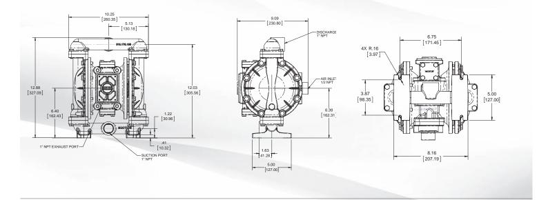
S1F Metallic - ANSI Flange Dimensions in inches (mm dimensions in brackets). Dimensional Tolerance:±1/8" (± 3mm) The dimensions on this drawing are for reference only. A certified drawing can be requested if physical dimensions are needed.
