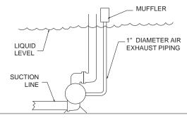
Pump can be submerged if the pump materials of construction are compatible with the liquid being pumped. The air exhaust must be piped above the liquid level. When the pumped product source is at a higher level than the pump (flooded suction condition), pipe the exhaust higher than the product source to prevent siphoning spills.
