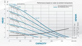
Max Capacity 150 GPM (568 LPM)
